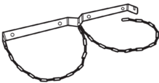
Fig. 13: Securing the gas cylinder
