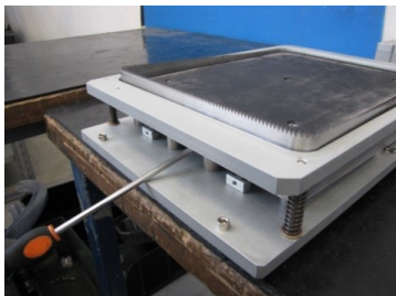
Fig. 40: Lifting out the cutting die
