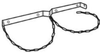
Fig. 11: Securing the gas cylinder
