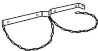
Fig. 10: Securing the gas cylinder
