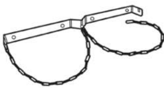
Fig. 10: Securing the gas cylinder
