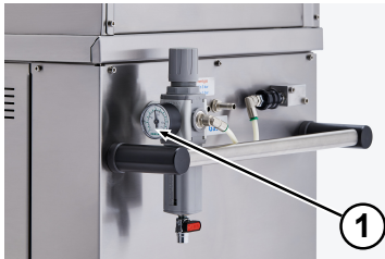
Fig. 18: Compressed air gauge
