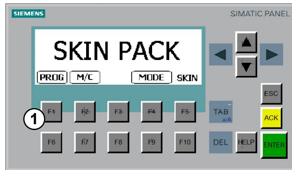
Fig. 8: Set sealing temperature
