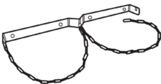
Fig. 28: Securing the gas cylinder
