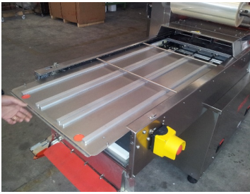
Fig. 71: Removing the loading area
