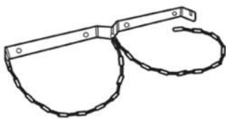
Fig. 9: Securing the gas cylinder
