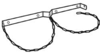
Fig. 9: Securing the gas cylinder
